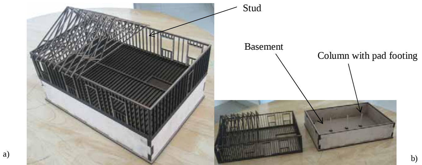
Photo 6: Wood Light Frame (WLF) Platform Construction Model (a). Basement and 1 st floor is not connected to clarity (b). Photo by Vaid
